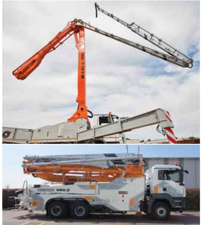
Carbon fiber booms replace steel in the final sections of the mechanical arms mounted on trucks like this one to place pumped concrete in hard-to-reach locations.
