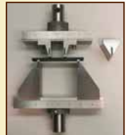
Three and Four Point Flexure ASTM D 790, D 6272, D 7264
