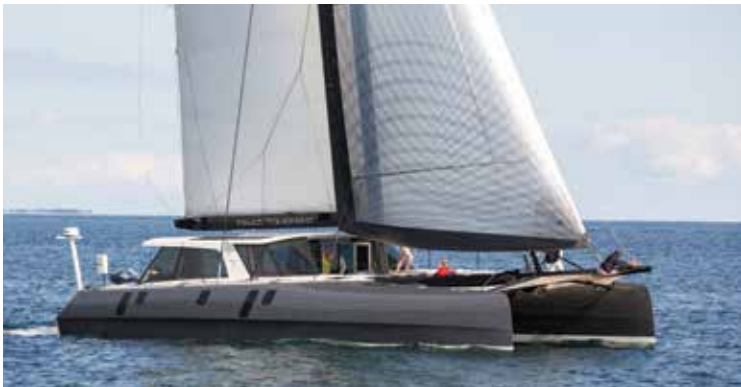
Gunboat International's 78 catamaran features a one-piece deck, molded from composites. Pictured is the smaller Gunboat 60 of similar design. Source / mouldCAM
