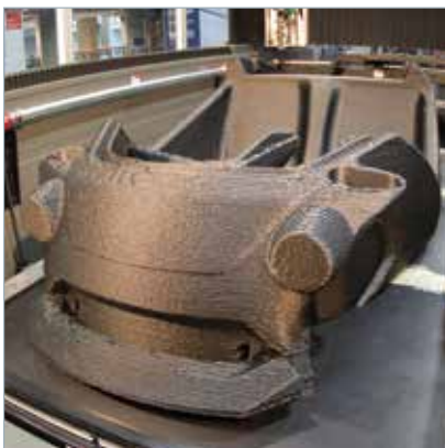
3 Here, BAAM builds up the laminate in 212 layers to form the car's main structure, including frame, seats, cockpit, hood and tail.
