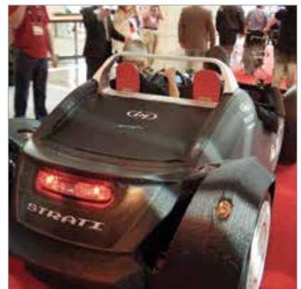
9 Finally, Strati is outfitted with windshield, roll bar, lights and seat covers.
