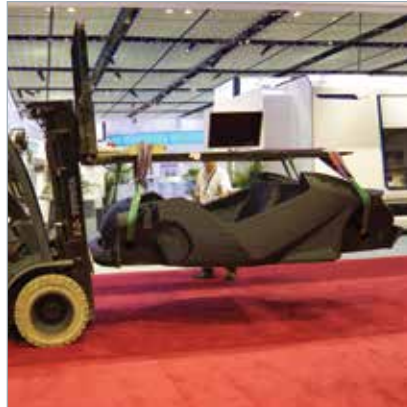
4 At only 454 kg, the printed CFRP tub is easily transported to another booth on the IMTS show floor for machining.
