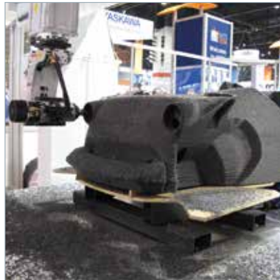
5 The tub is machined where surfaces require smoothness and tight tolerances for mating parts, using a Thermwood Inc. (Dale, IN, US) 5-axis CNC router.
