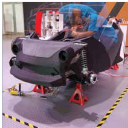
6 The machined tub is returned to the exhibit booth for further assembly.
