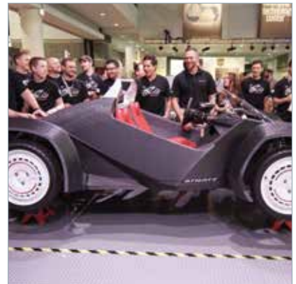
8 Strati's fenders, printed separately on BAAM and machined, went on over the wheels.
