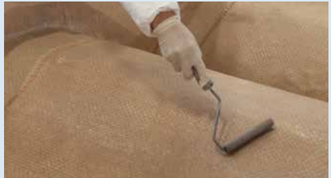
4 An impregnator was used to wet out three plies of glass fiber woven roving for each panel, which were then applied to and rolled out on the molds by hand.
