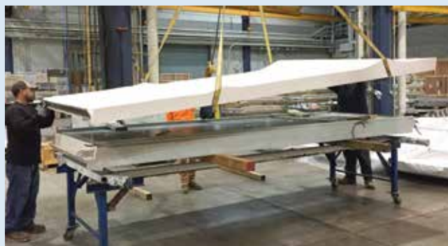
7 At the Enclos facility, technicians assembled each unitized wall system panel for the SFMOMA expansion, and then attached the matching Kreysler FRP rain screen panel, like the one shown here as it is lowered onto an Enclos wall system panel. Source (Step 7) | Enclos
