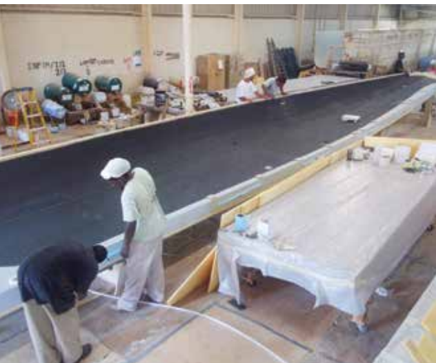
Gold Coast workers tend to a partially layed-up B53 hull section in preparation for eventual bagging and infusion. Source | FORMAX
