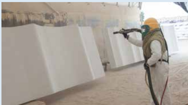
6 Sandblasting the gel coat to reveal the desired matte finish was the final step before shipping the panels to Enclos.
