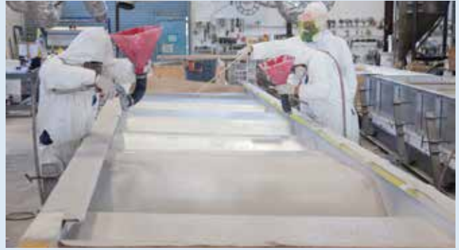
3 After applying the mold release, Kreysler technicians sprayed on the Fireshield 285 coating.
