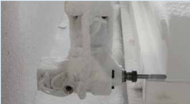
2 Molds were CNC-machined from EPS foam.
