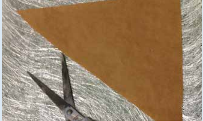
3 The reinforcement is hand cut, using paper templates, then layed up into the tool.
