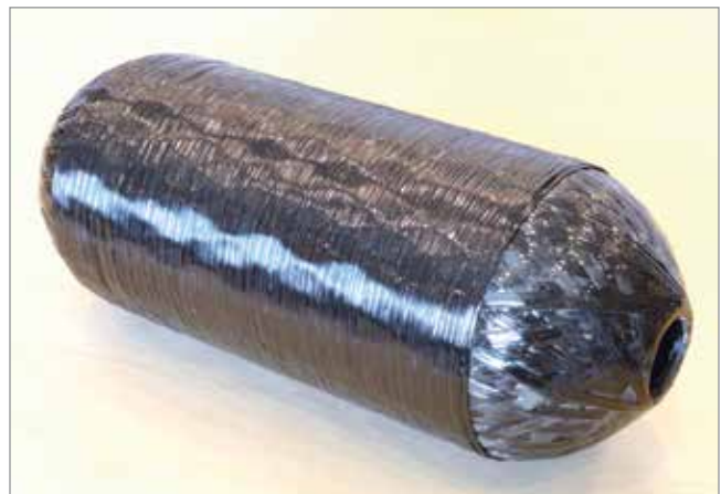
FIG. 4: Washout mandrels for pressure vessels
