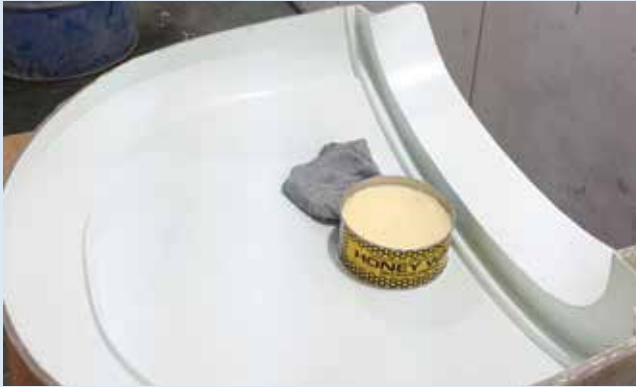
1 Single-sided composite tooling receives a coating of wax prior to start of layup.
