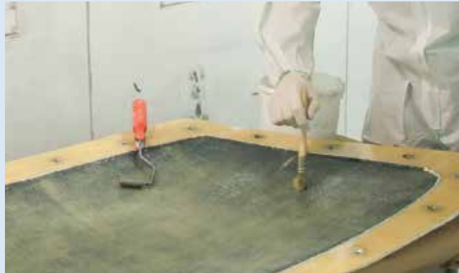
4 When each layer of reinforcement is in place, unsaturated polyester resin is carefully hand applied in a laminating step. The goal is to avoid adding too much resin, which otherwise could cause cracking. During this step, flanges and other hardware are also bonded into parts.
