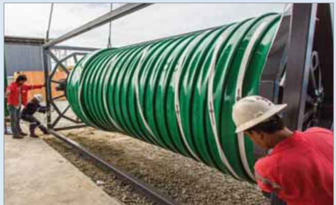
3 After the liner cools and the thermoplastic layers solidify against the core, the liner is reeled onto a transportation drum in a flat configuration.
