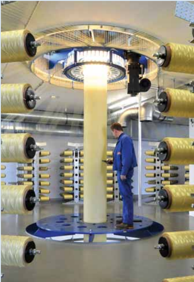
1 A single-ply, 2-mm-thick cylindrical structure is woven from Kevlar. The aramid fiber is drawn from hundreds of spools and woven in a manner similar to sock knitting, in (as shown) vertical format. Source (all step photo) | APS
