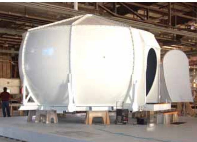
Designed by Pagnotta Engineering Inc. and built by JRL Ventures, this projection dome for CEAL's driving research simulator met all technical, weight and cost requirements, using fire-retardant, resin infused composites. Source | PEI & JRL Ventures
